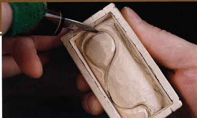
STEP 13 Using the knife, further define the v-groove first by plunge cutting...
