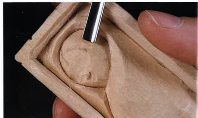
STEP 18 Using a 1/4" shallow gouge, create a hollow representing the nose bridge and eye area. Keep it very shallow!
