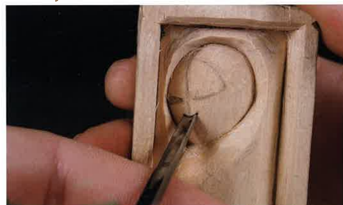
STEP 17 Using a 1/8" shallow gouge, plunge straight in where the nose will be. Refer to the pattern for placement.
